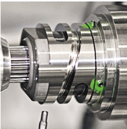
Figure 5: Interchangeable slide piece with endless guide
