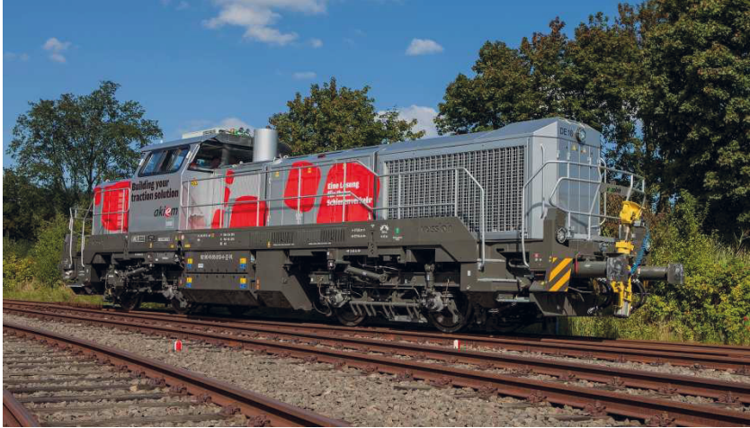
Figure 3: Vossloh's new multipurpose diesel locomotive with MTU 12V4000R84 diesel engine
