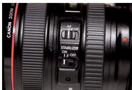
Figure 1-8: Slide this switch to enable image stabilization.
