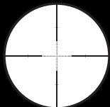
TMR, Tactical Milling Reticle
